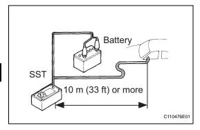
(2) Connect the SST connector to the airbag connector of the spiral cable.
