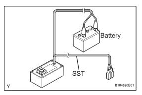
(1) Connect SST to the battery. Connect the red clip of SST to the positive (+) battery terminal and the black clip of SST to the negative (-) terminal.
